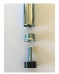
**1.** Remove the foot and insert from the bottom of the post by simply unscrewing both pieces.
