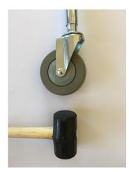
**3.** If needed, tap the castor with a rubber mallet until fully inserted.
